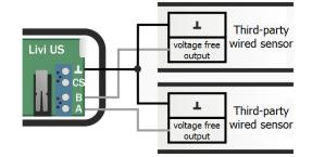
If you want to connect only one third-party wired sensor to the device, use the following connection diagram:
