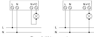
Figure 2: Wiring examples
