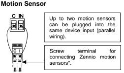
\* In case of using ZN1IO-DETEC-P sensor, its micro switch number 2 must be in **Type B position**.
